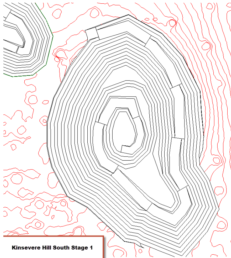
Figure 44 Kinsevere Hill South Pit Design
