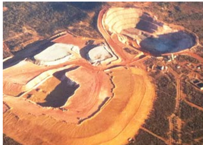
Figure 67 Aerial view of open pit and waste dump development
