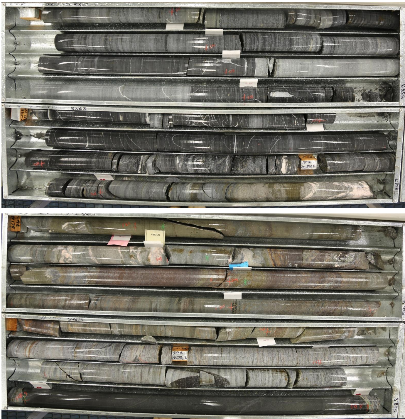
Figure 12. Polymetallic mineralisation intersected in 519R at the AB- North target, 60m north of known mineralisation.
