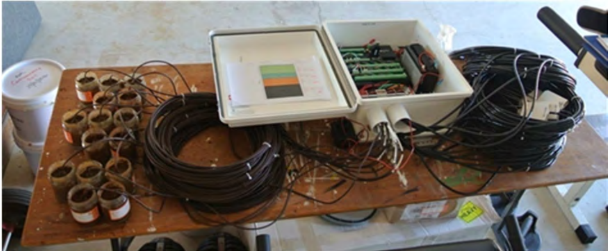
Photograph 3 Matrix suction sensor calibration
