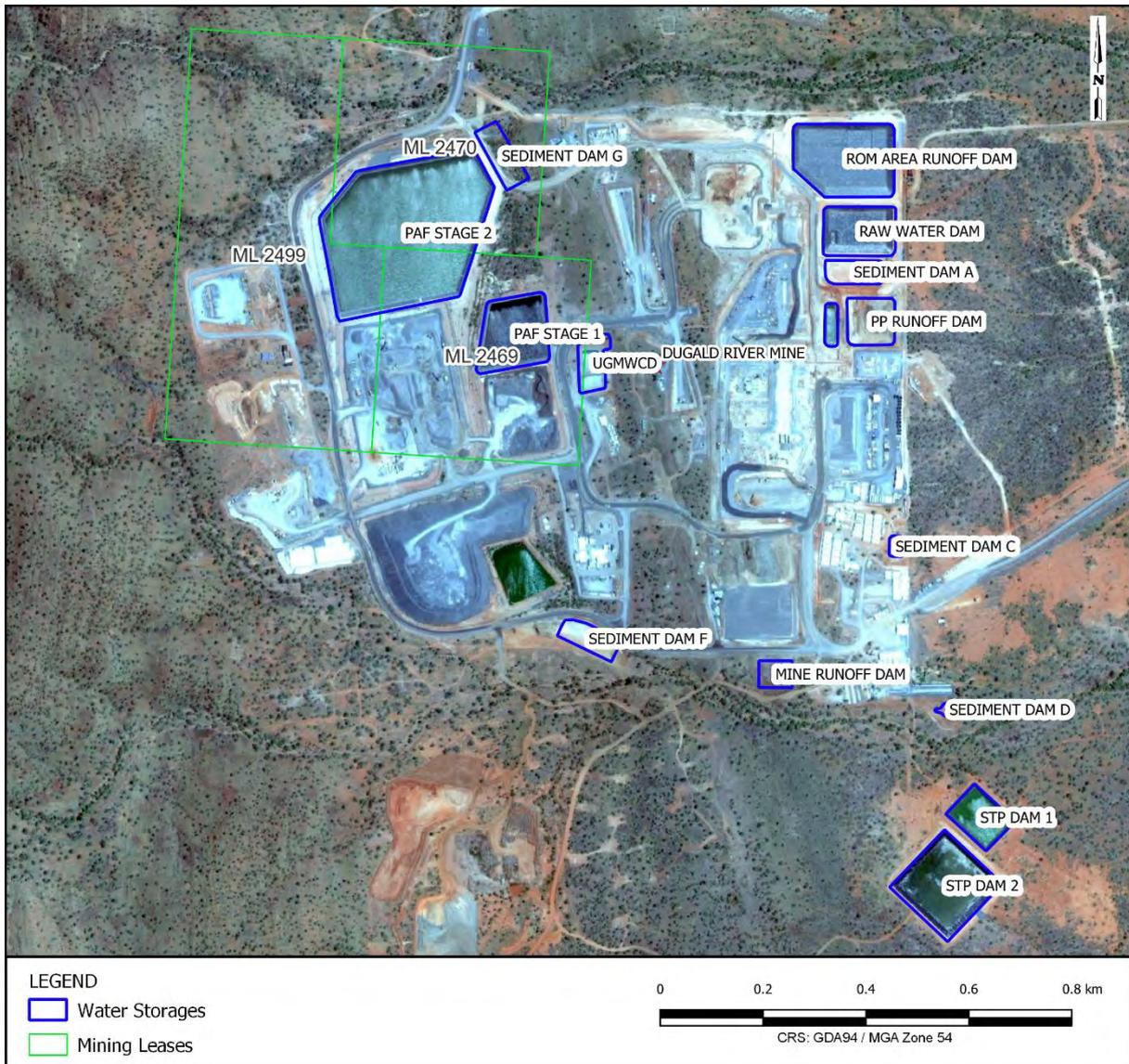
Waste rock materials from the underground mining operations are stockpiled on dedicated, non-acid forming (NAF) and potentially acid-forming (PAF) pads.
