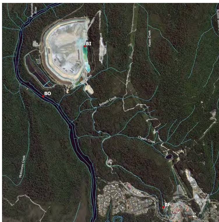
Figure 4-1. Internal monitoring locations BF (head of Flume) and BI (Bobadil intermediate). The discharge point BO is also indicated.
