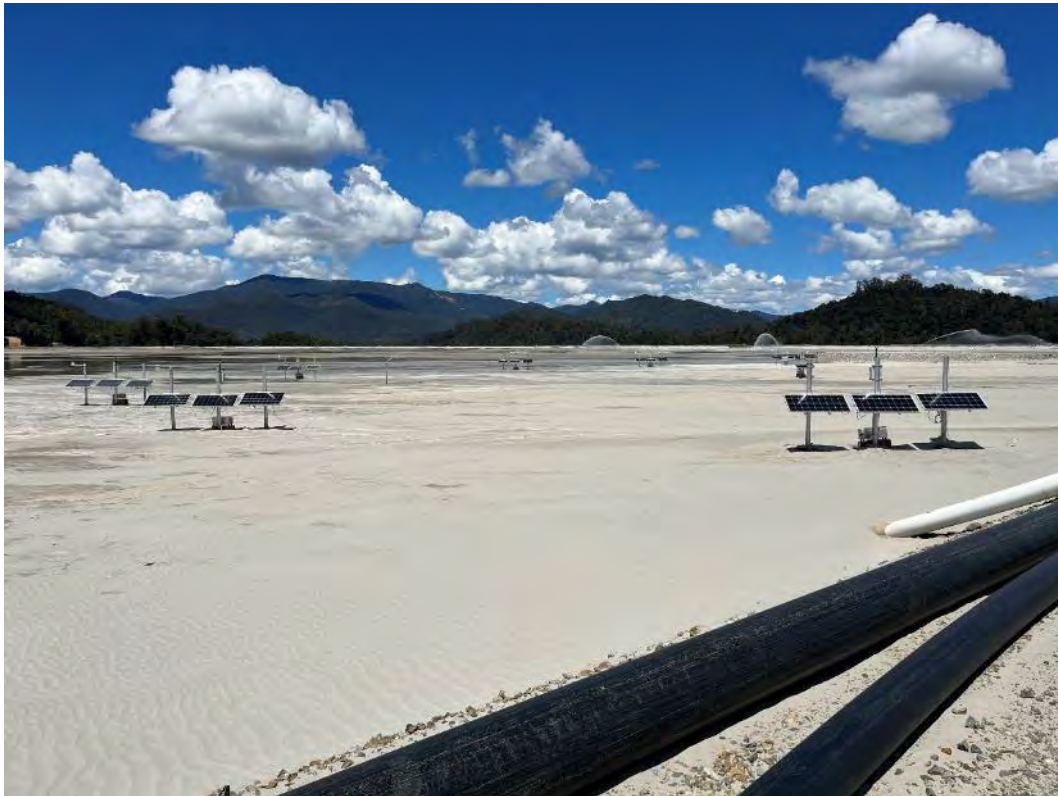
Photograph 27 – Dust monitoring equipment on tailings beach near levee embankment.
