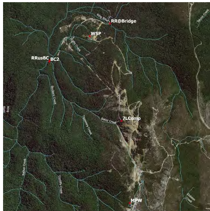
Figure 9-1. Surface water monitoring locations at the Hercules Mine site. Monitoring site Ring at Highway (RAH) is located downstream on the Ring River at the Murchison Highway, north of the extent of the photo.
